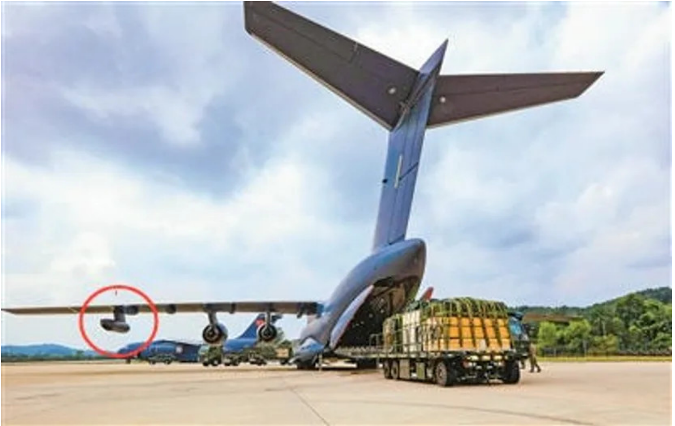
(Cargo being loaded into a Y-20B MRTT. Refueling pods have been circled in red. Image Source: PLA Daily. 14 Oct 2026)
